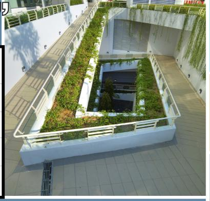
The continues vegetation connects the green area from Level 1 retail garden down to Basement 2 level, and channels surface rainwater into a drain at Basement 2 then will be pumped up back to ground level.
